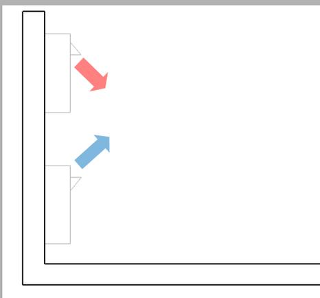
As optional is possible to supply only for WZ-32 a fixed flap useful for high wall installation to push the hot air down or to push cold air in high position and not against the people .
