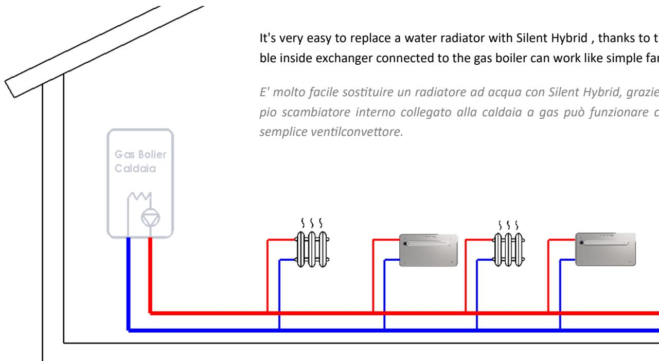
It's very easy to replace a water radiator with Silent Hybrid , thanks to the double inside exchanger connected to the gas boiler can work like simple fan coil .
