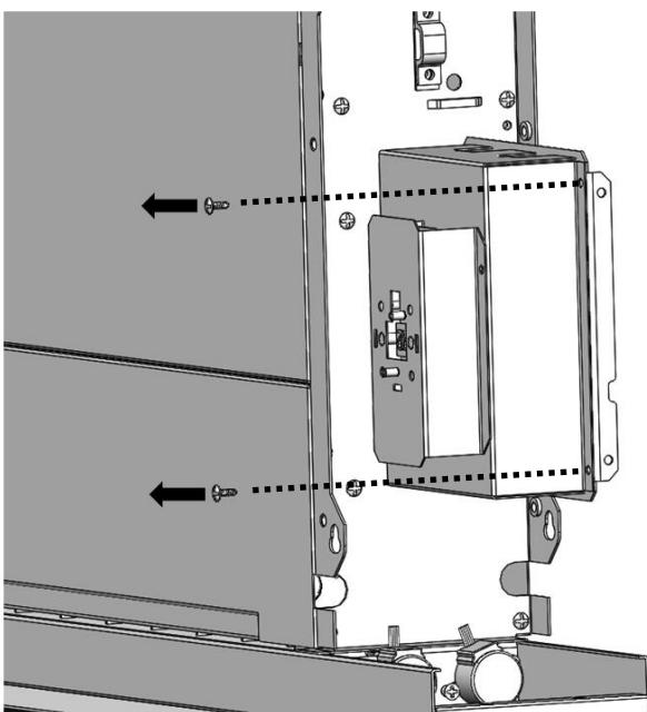
To access to main PCB, remove the two screws shown in the picture on the left
