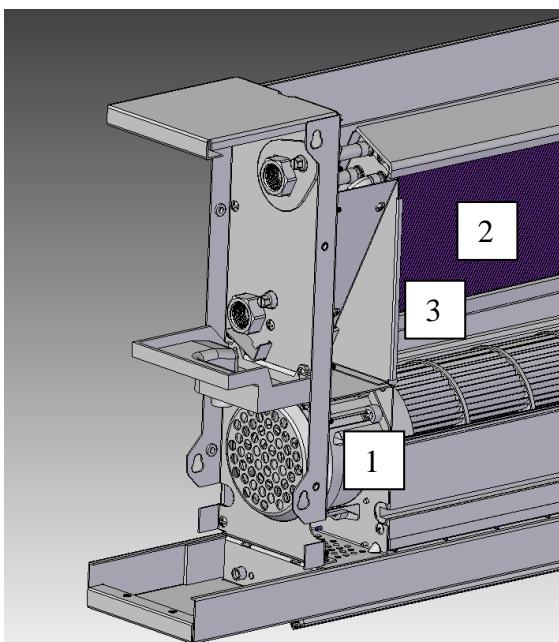
Remove the two front panels. See page 7 for exploded view.
