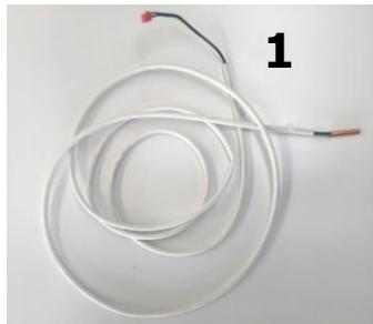
The water probe is used as minimum and maximum sensor. It must be positioned by the installer in the coil brass cylinder, near the copper pipe in proximity to the Inlet of the same coil. The probe must measure the water temperature sent to the external unit. The probe must be connected in the main electronic board as indicated.
