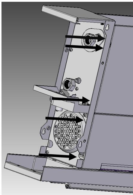
To access internal components, remove screws on both the sides of the two front panels, as indicated in the picture on the left.
