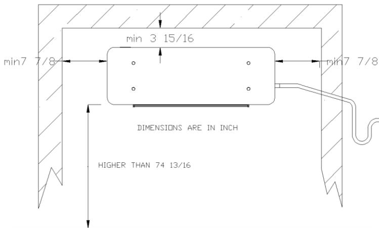
Position the unit on a structure able to support its weight. We recommend the use of antivibration systems to prevent the transmission of vibration to the supporting structure.
