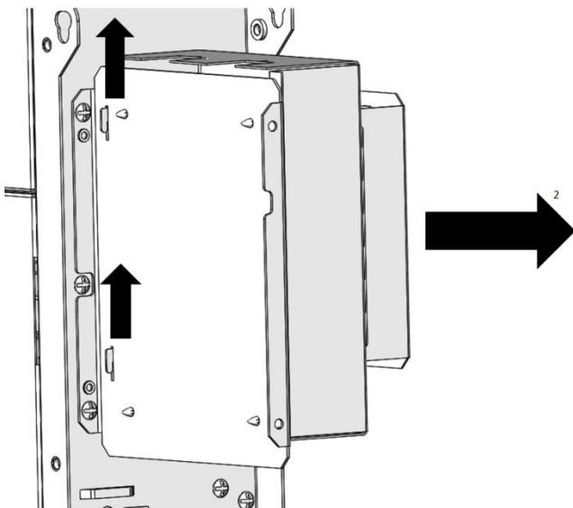
To remove the cover and access to main PCB, slide the assembly up to release from its bracket.
