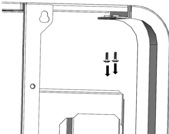
Remove the two top screws and remove the right side panel. Remove the two top screws at the top of the left panel and remove the panel.
