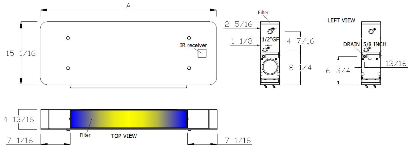
Standard configuration is to provide right hand hydronic connections from the factory.
