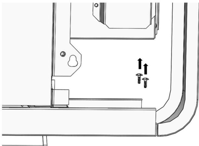
Remove the two bottom screws on the right side panel.. The left side panel will have two bottom screws as well.
