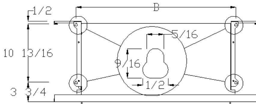
Drill mounting holes in accordance with dimensions shown in the above figure. Determine appropriate anchors to use and attach mounting bracket to the wall. Attach fan coil unit to bracket.
